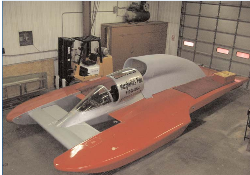
Here's what Tubby looked like in mid-June. Notice the new cowling has been built and placed for fit. Guess who's providing the pizza for work crews.
