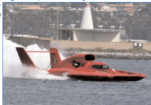
The U-3 wears a cowling over the turbo Allison during its second qualifying run in San Diego, results were worse with the cowling on than off.
